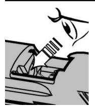
Removing cartridges from the magazine does not prevent the pistol from being fired! When there is a cartridge in the chamber, the cartridge will discharge if the trigger is pulled. It is absolutely essential for the user to know how to completely unload the pistol. "Completely" means emptying the magazine and removing a chambered cartridge.
